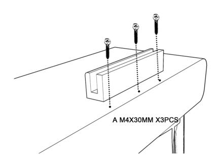
MOUNT THE MIRROR SUPPORT TO THE TABLE AS SHOWN, USING SCREWS A(X3PCS).
