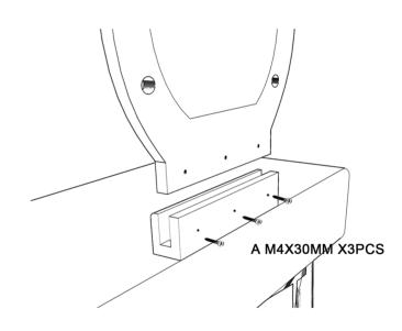
INSERT THE MIRROR INTO THE MIRROR SUPPORT AND FIX IT WITH SCREW B(X3 PCS)
