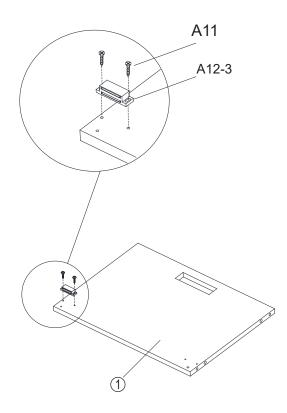
Note: According to your needs, the door can also be installed on the other side in the same way.
