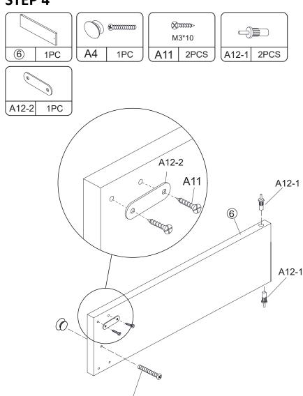
Note: According to your needs, the door can also be installed on the other side in the same way.
