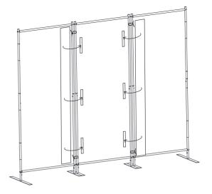
Secure the two adjacent pillars with straps, Then cover it with Velcro
