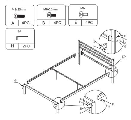
Joing part 6 and part 4/5, using bolt A, bolt B, Nut E with Allen key F Joing part 1/2, part 3, part4/5, using bolt A, bolt B, Nut E with Allen key F
