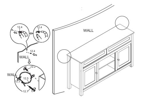
Follow the instructions printed on the plastic bag containing the tipping restraint hardware to attach thetip-over restraints to the unit and the wall.
