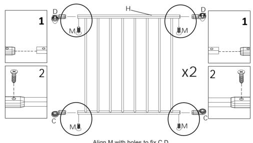
Align M with holes to fix C,D.
