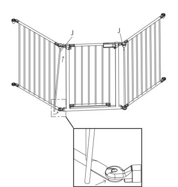
please adjust the angle before installing the steel bar
