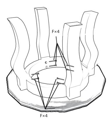
Do not screw all the screws when installing the table legs and stool legs. Keep half-screw state until all installation adjustments are complete before screwing the screws.
