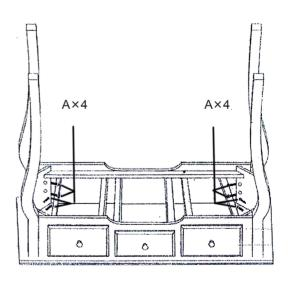
Do not screw all the screws when installing the table legs and stool legs. Keep half-screw state until all installation adjustments are complete before screwing the screws.
