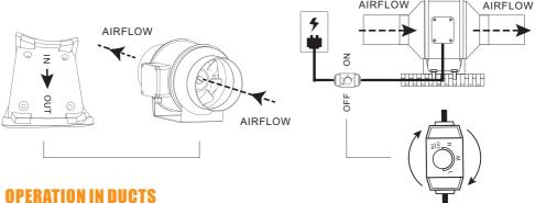
This booster fan fits standard 4 inch.6 inch and 8 inch air ducts
