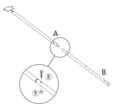
Screw the bolt into the small threaded hole to connect (A) with (B).
