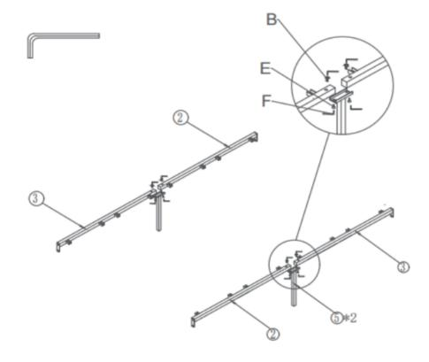
Connect part 2 and part 3 through part 5, using bolt B, Nut E with Allen key F
