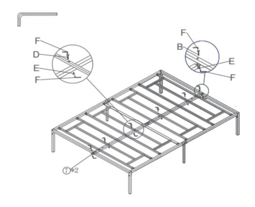
Connect part 4 and part 2/3, using bolt C with Allen key F
