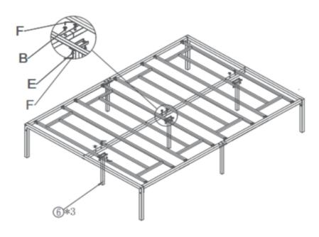
Connect part 6 and part 7 together, using bolt B, Nut E with Allen key F
