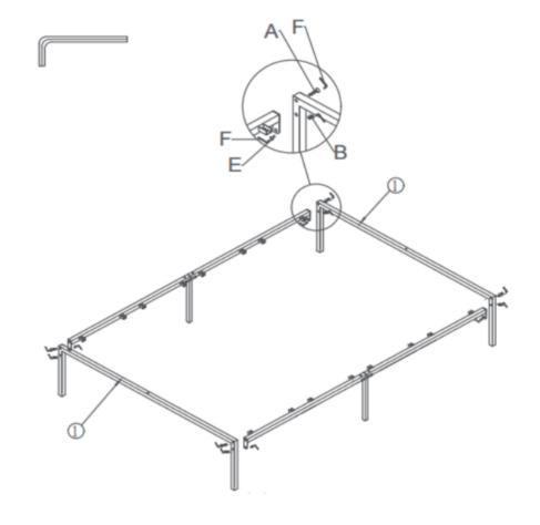
Connect part 1 and part 2/3/5 together, using bolt A and B, Nut E with Allen key F
