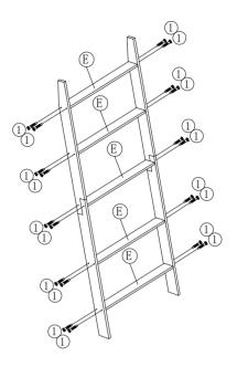
Keep half-screw state until all installation adjustments are complete.
