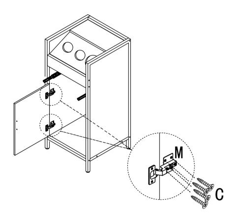
The distance between the door and the side panel canbe adjusted by the hinges.
