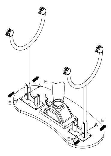
**First**: **Remove the screws E** (Put the screws in place for next use)
