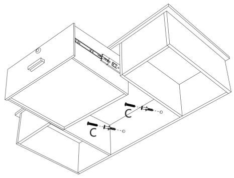
The cabinet hardware C (X 2SETS) is loaded into the wall(as shown above).
