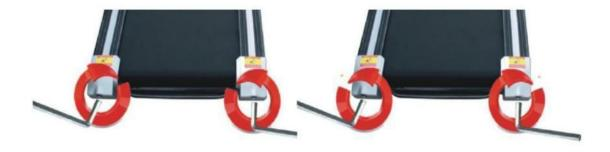
Please adjust the left bolt clockwise or adjust the right bolt counterclockwise if it's left deviation. And implement the contrary measures if it's right deviation.
